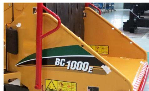
**A LARGE RECTANGULAR 12 IN X 17 IN (30.5 CM X 43.2 CM) FEED OPENING.** Helps with productivity by reducing the need to trim material before feeding it into the chipper.
