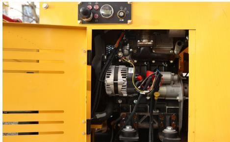
**25 HP (18.4 KW) EFI ENGINE.** Performs well during cold-weather starts, minimizes occurrence of engine flooding and provides improved fuel economy over comparable carbureted diesel engines. Gas engine option also available.
