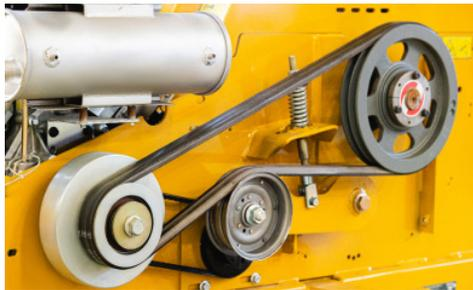
**THE CENTRIFUGAL CLUTCH.** Helps prevent belt-slip when engaging the clutch to minimize maintenance.
