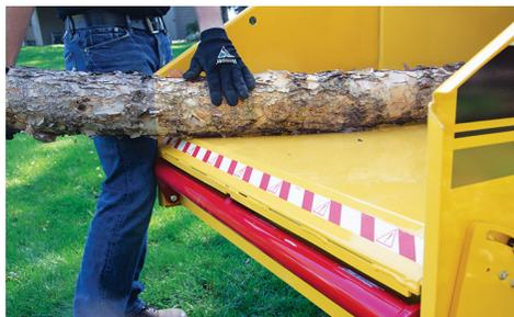
**BOTTOM-FEED STOP BAR.** Is strategically located to make it possible for an operator to strike the bar and shut off the feed mechanism.
